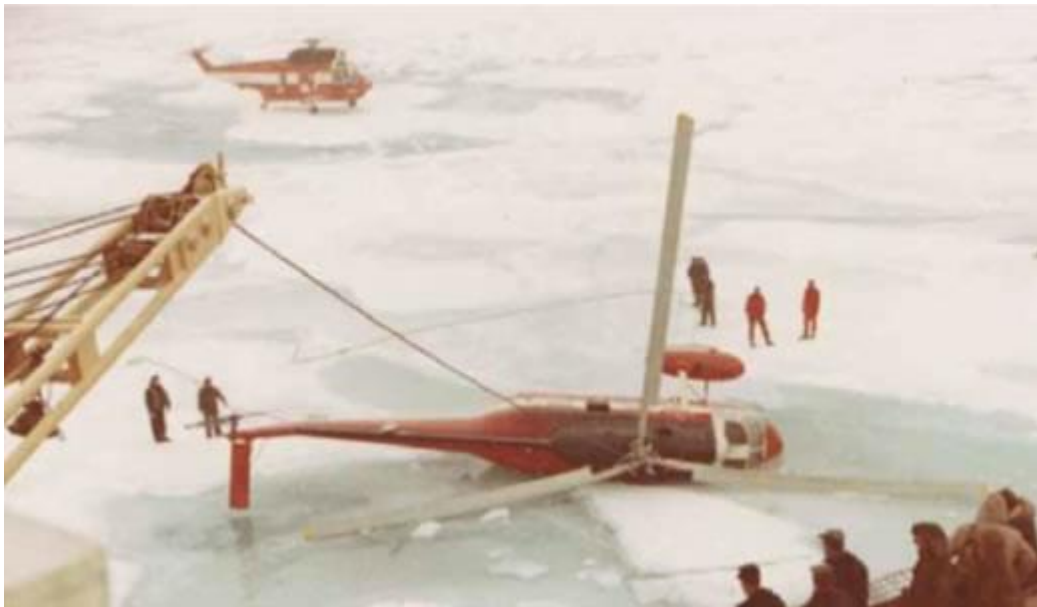
Recovering a helicopter which landed with one wheel on a hole in the ice.
