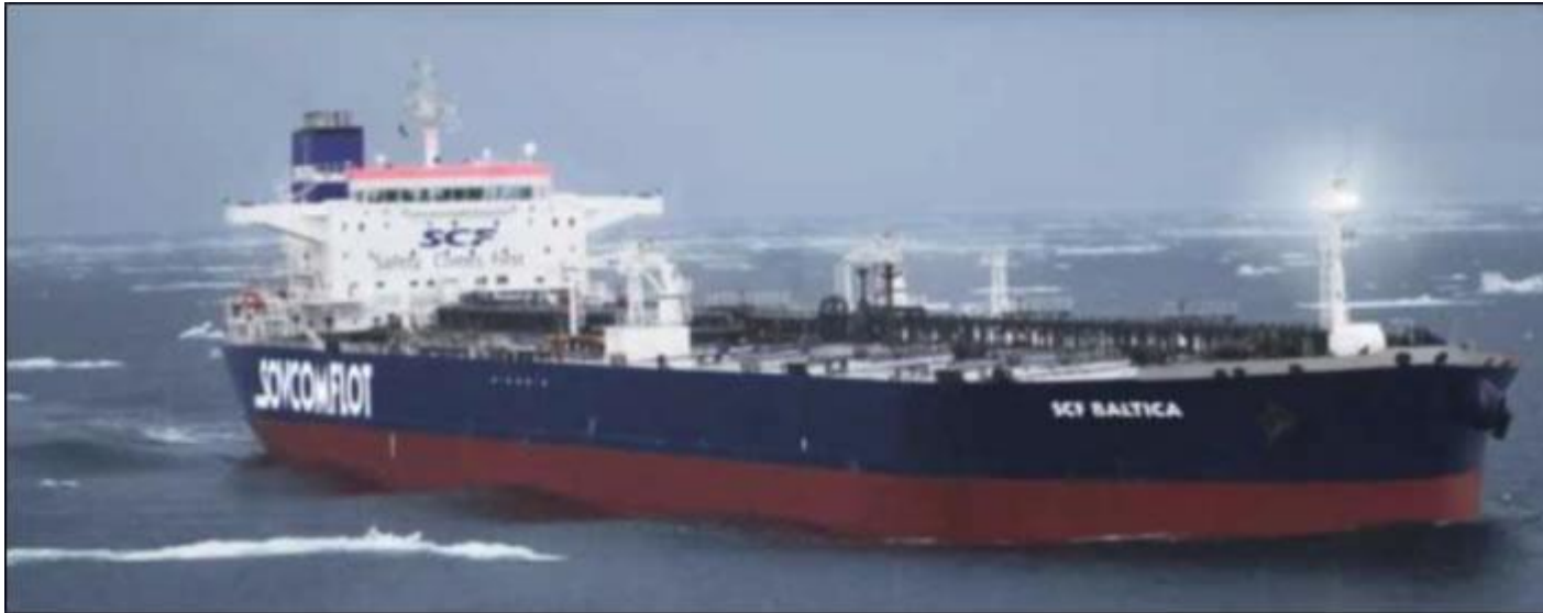
The Arc5 oil tanker SCF BALTICA sailing in dispersed ice in the Laptev Sea. (Source: OAO Sovcomflot)
